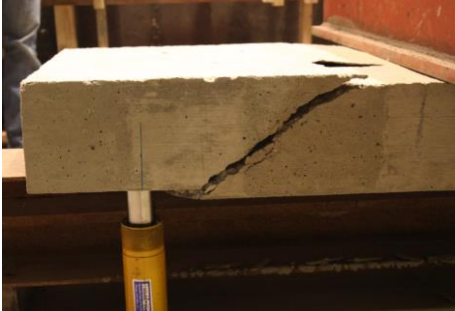
Figure 28. A photograph of the side view of the first peeling test (3 shear studs) (Dang 2013)
