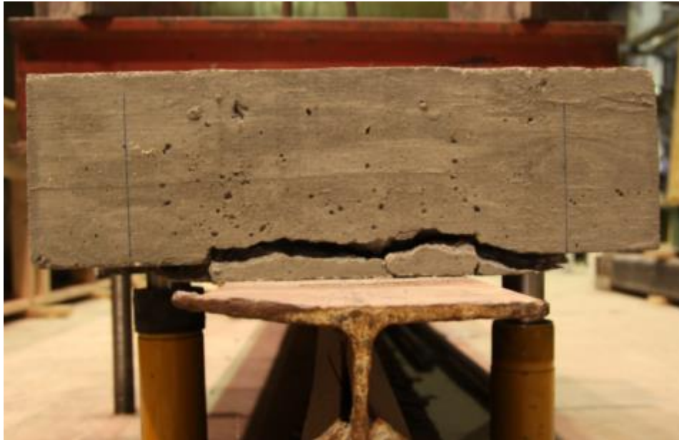
Figure 27. A photograph of the front view of the first peeling test (3 shear studs)
