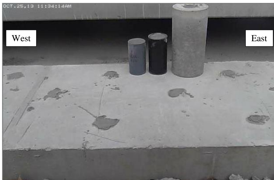
Figure 17. A photograph of the chemical splitting specimen and the grout
