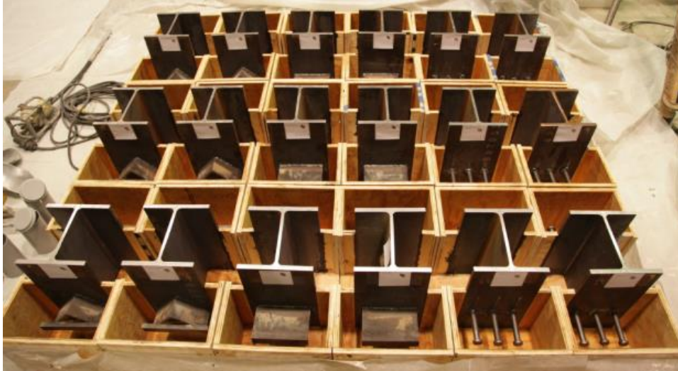
Figure 38. A photograph of constructed steel specimens and concrete formwork (Dang 2013)
