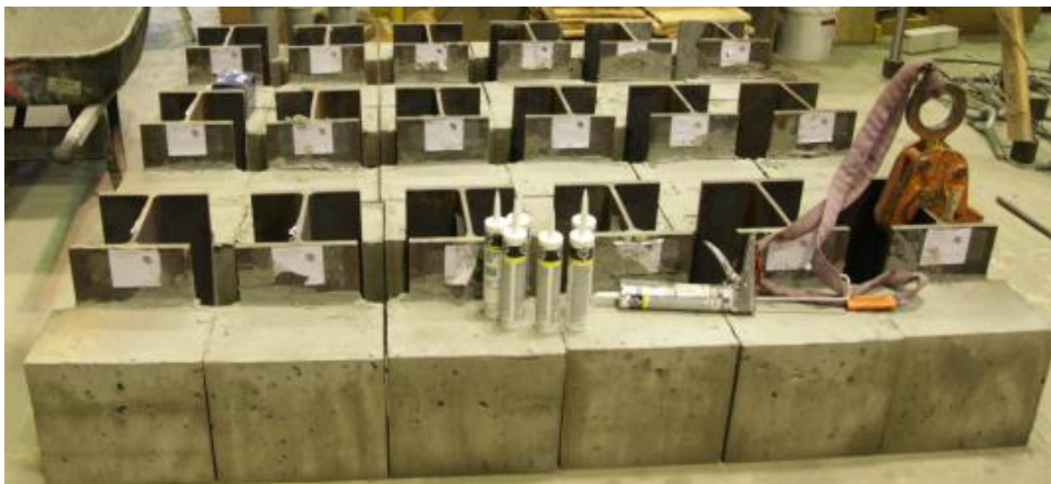
Figure 39. Eighteen specimens after initial concrete placement (Dang 2013)
