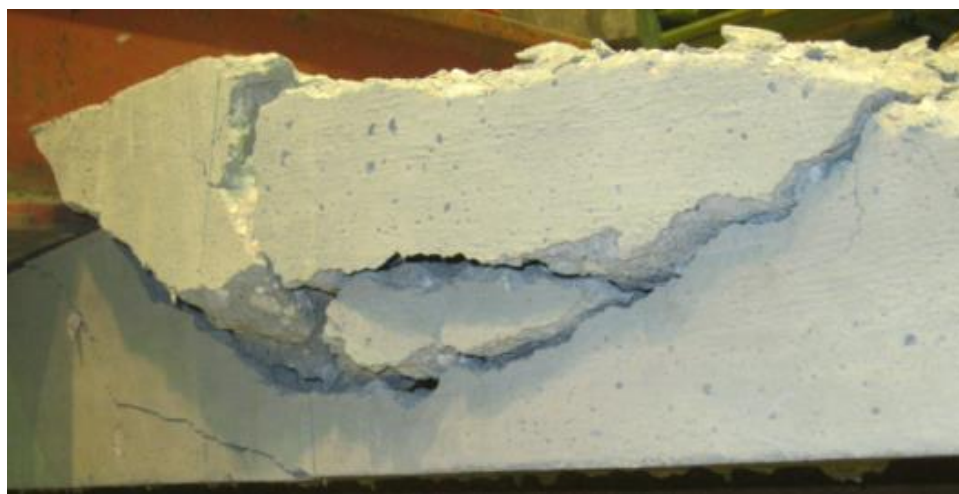
Figure 32. A photograph of fifth peeling test (3 shear studs) (Dang 2013)
