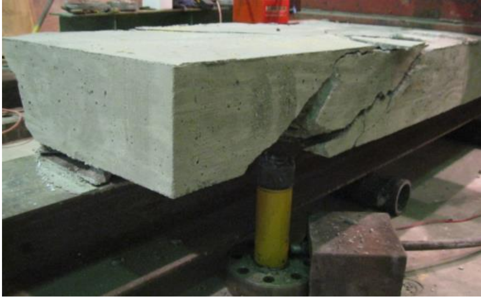
Figure 33. A photograph of the side view of the first peeling test (2 shear studs) (Dahlberg 2014)
