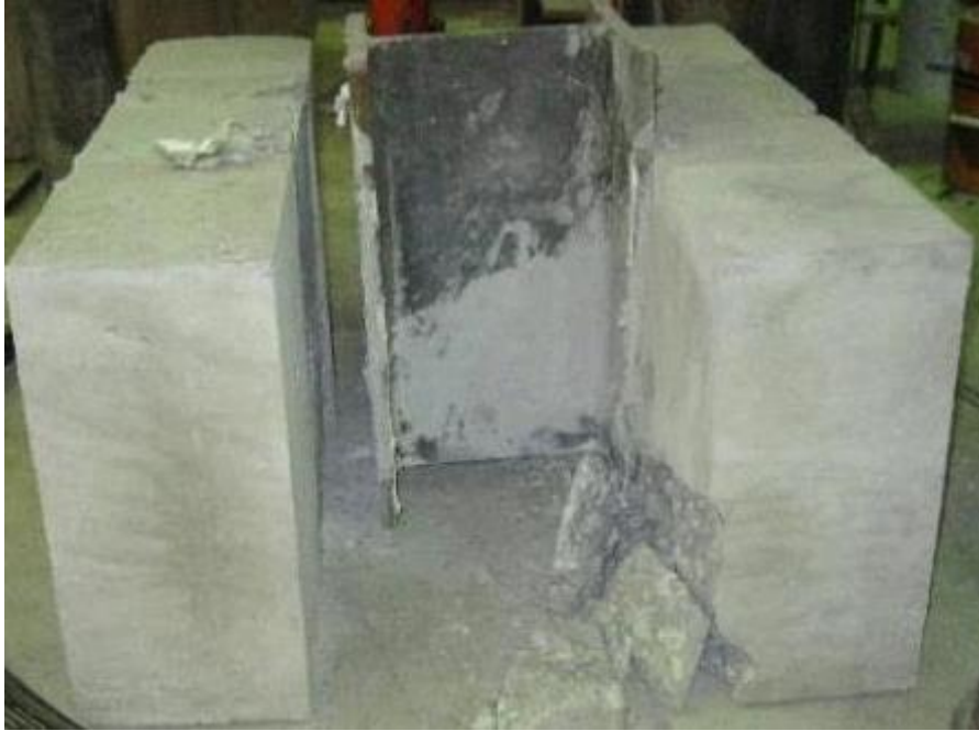
Figure 45. A photograph of shear connector failure (Dang 2013)
