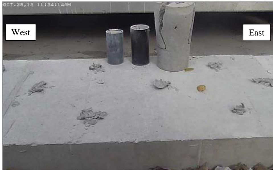
Figure 21. A photograph of the chemical splitting on day four (after 96 hours)
