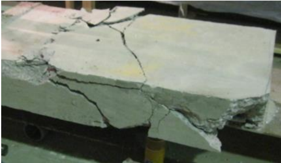
Figure 34. A photograph of the top view of the first peeling test (2 shear studs) (Dahlberg 2014)
